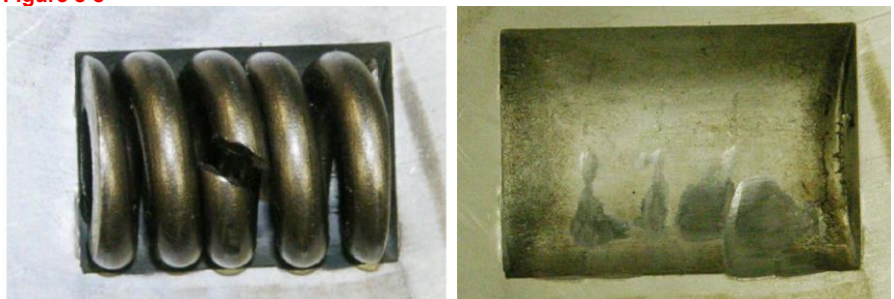
Broken damper spring and damaged deepening for damper spring
