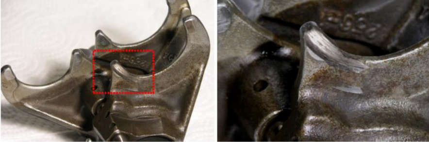
Gear shift fork for shifting the first gear with material wear at the ends
