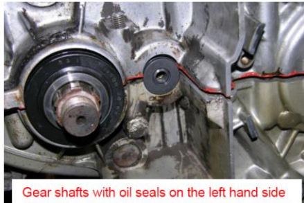
Gear shafts with oil seals on the left hand side
