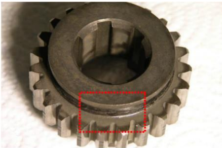
Gearwheel of the fourth gear on the transmission drive shaft
