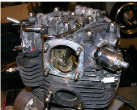
Install the cylinder head cover and the oil delivery pipe
