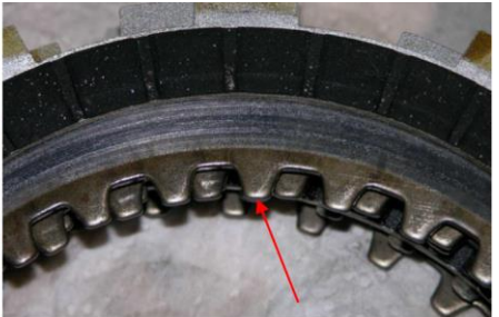
Insert the clutch discs - rounded side to the outside
