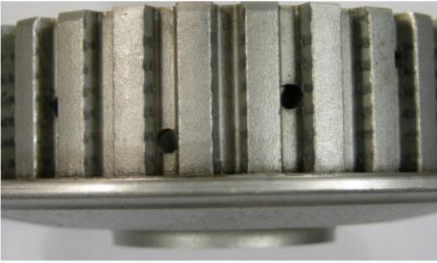
Clutch boss with imprints of the clutch disks
