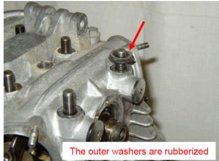
Loosen the bolts of the cylinder head
