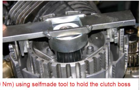
Assemble washer, belleville spring and nut
