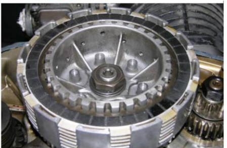
Insert the clutch discs - rounded side to the outside
