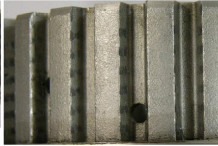
Clutch boss with imprints of the clutch disks
